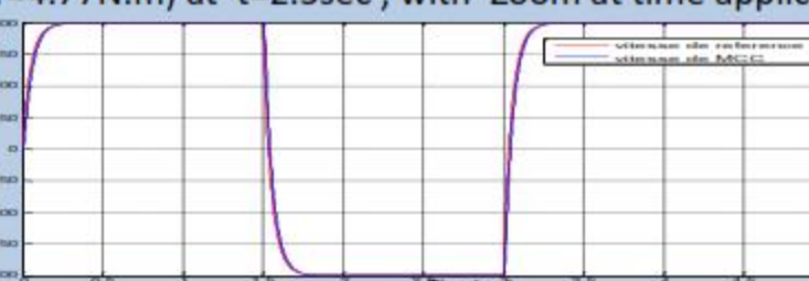
Fig.4. speed response (rad/sec)/time(sec), Reversing the direction of rotation .
