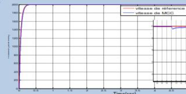
Fig. 3. Speed response(rad/sec)/time(sec) start with no load and application load (Cr=4.77N.m) at t=2.5sec, with Zoom at time application load.
