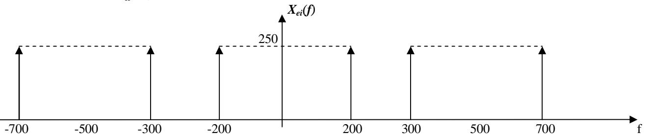
**Conclusion :** The right choice of sampling frequency  $f_e > 2f_{\max}$ , Shannon's theorem respected, does not give a spectral folding which allows us to recover the signal
