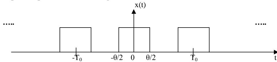
b.  $x(t)$  is it a finite mean power signal ( $P_x < \infty$ ) ;  $x(t)$  is a periodized signal (unbounded support represented by the dots .... )
