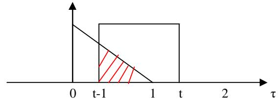
2. The convolution product expresses the amount of overlap of a signal  $x_2(t)$  when moved to another signal  $x_1(t)$
