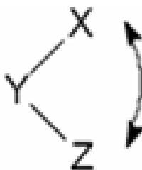
Figure III.6. Angular deformation (variation of the angle between two adjacent bonds).
