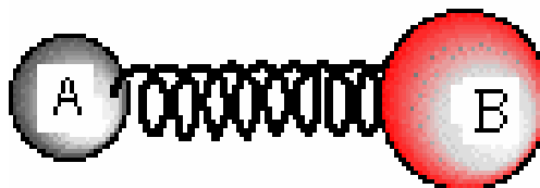
Figure III.1. Comparison of the vibration of two atoms linked by a chemical bond to that of two balls of masses m_A and mass m_B connected by a spring.
