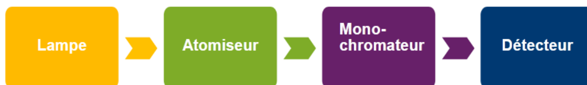
Figure V.3. Schematic diagram of an atomic absorption spectrometer device
