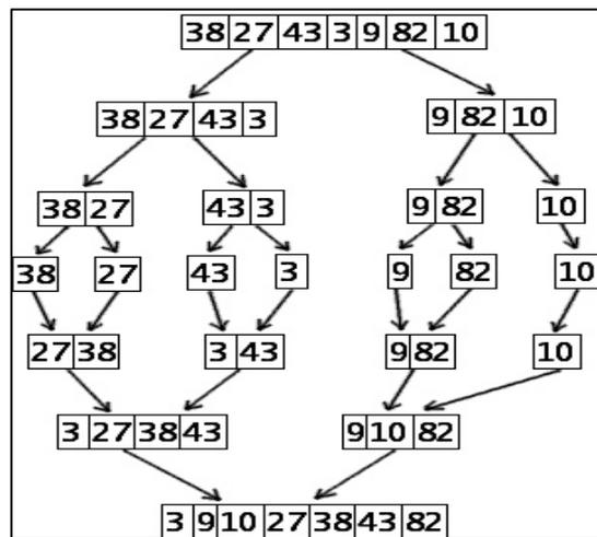
**Figure 2.2.** Sorting array  $T$  using merge-sort algorithm.
