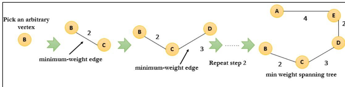
**Figure 1.4.** The resulting minimum spanning tree using Prim's algorithm.
