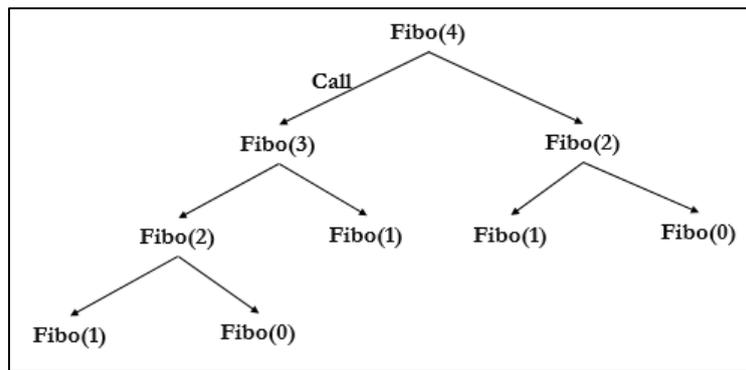
**Figure 3.1.** Execution scheme of Fibonacci sequence by the divide-and-conquer method.
