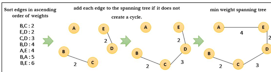
**Figure 1.5.** The resulting minimum spanning tree using Kruskal's algorithm.
