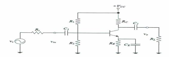
Assume that: VCC = 15 V,  $\beta = 150$ , VBE = 0.7 V,  $RE = 2.7 \text{ k}\Omega$ ,  $RC = 4.7 \text{ k}\Omega$ ,  $R1 = 47 \text{ k}\Omega$ ,  $R2 = 10 \text{ k}\Omega$ ,  $RL = 47 \text{ k}\Omega$ ,  $Rs = 100 \Omega$ .
