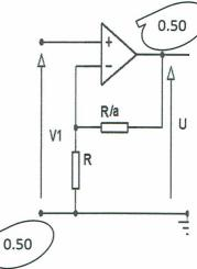
$$0.50 \quad \gamma_1 = V^- = \frac{R}{R + R/a} U \quad \rightarrow \rightarrow \rightarrow U = \left(\mathbf{1} + \frac{1}{a}\right) V_1 \dots (1)$$
