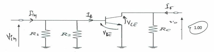
Replacing the transistor by its small-signal AC equivalent circuit, we have
