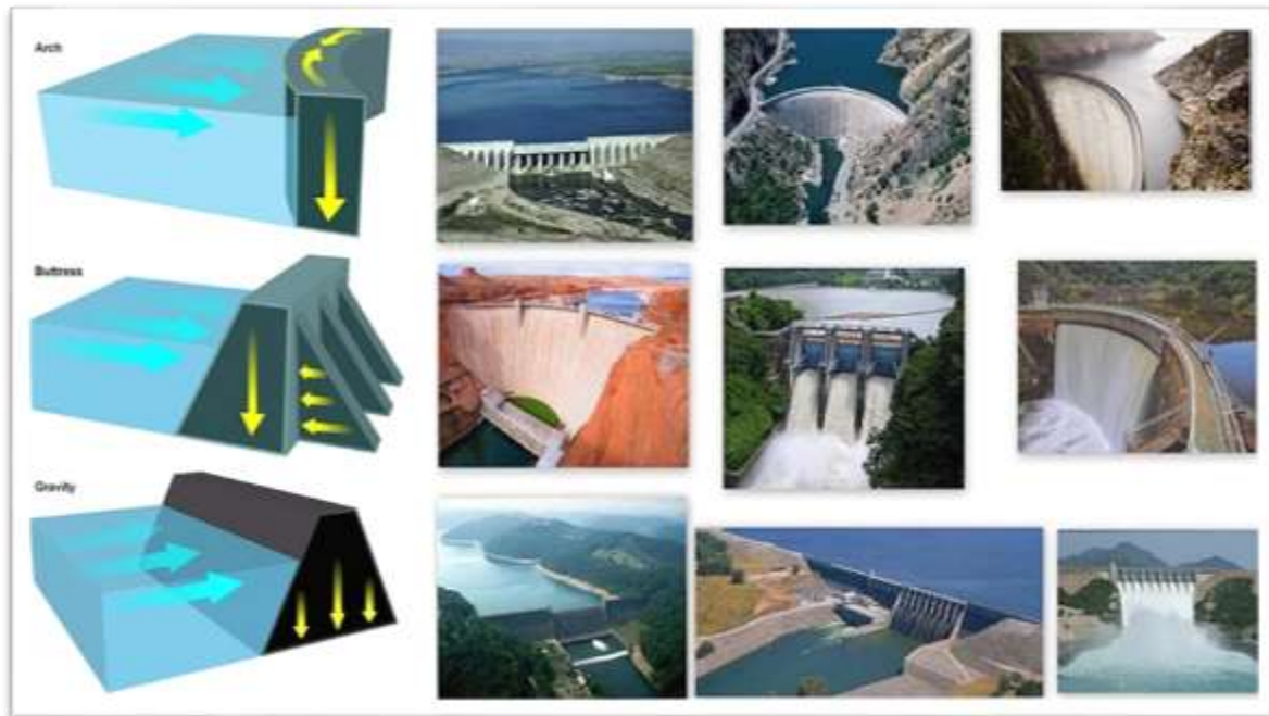
Figure 12 : Some types of rigid dams. Source: 12
