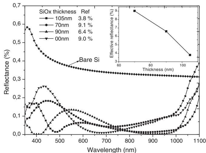
Fig. 4. Reflectance spectra of  $\text{SiO}_x$ /PS films on  $n^+/p$  junction for various thicknesses  $\text{SiO}_x$  (inset of plot: effective reflectance versus different  $\text{SiO}_x$  layers thicknesses).
