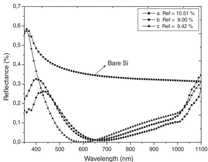
**Fig. 2.** Total reflectance spectra of: (a) PS growth in HF (48%):  $\text{C}_2\text{H}_5\text{OH}$ =3:1,  $J=20 \text{ mA/cm}^2$ ,  $t=6 \text{ s}$ ; (b) HF (48%):  $\text{C}_2\text{H}_5\text{OH}$ =4:1,  $J=20 \text{ mA/cm}^2$ ,  $t=6 \text{ s}$ ; (c) standard  $\text{SiN}_x$  ARC (73 nm).
