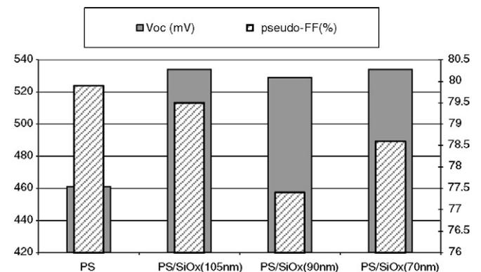
Fig. 5. Parameters suns- $V_{oc}$  obtained in a junction  $n^+/p$  with PS and PS/ $\text{SiO}_x$  as ARC.
