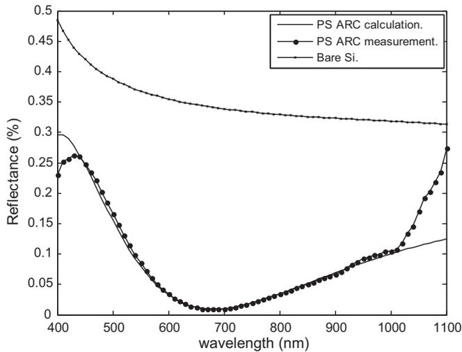
Fig. 3. Calculation and experimental reflectance spectra of PS layer ARC grown on  $n^+/p$  junction.
