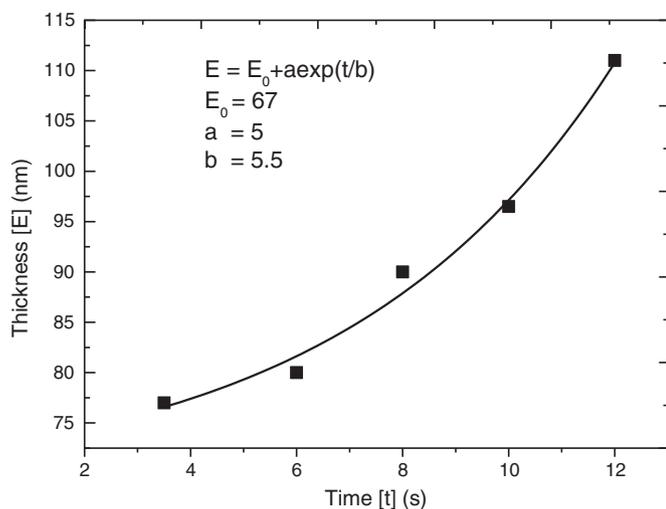
**Fig. 1.** Thickness  $E$  vs anodization time  $t$  of PS growth at a constant current density of  $20 \text{ mA cm}^{-2}$  on  $n^+$  diffused side of (100) Si wafer.
